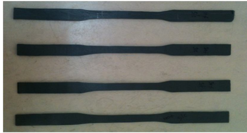
Fig2 Image of cast tensile specimens
